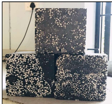
Fig 1: Polystyrene cube specimens
