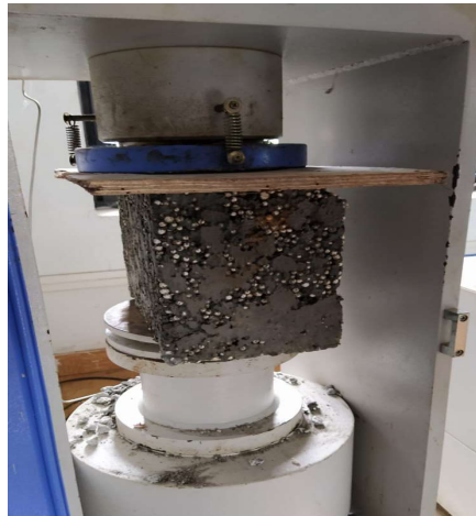
Fig 9 Compression Test on Polystyrene block
